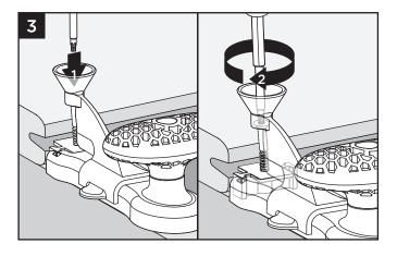
Using bit included with one-step tool, install screw as shown. Screw should be slightly countersunk into fastener when installed correctly. Continue to install fasteners on every joist. Do Not Overdrive Screw.
