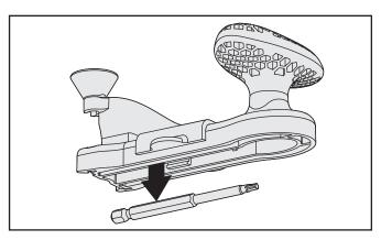
Only use bit that is supplied with one-step tool, using a different bit will not allow tool to work correctly or allow fasteners to seat correctly. Bit is conveniently located on the underside of the one-step tool. For replacement bits please visit Shop.Trex.com.
