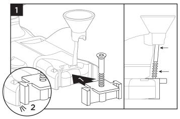
Place Hideaway hidden fastener into one-step tool.
