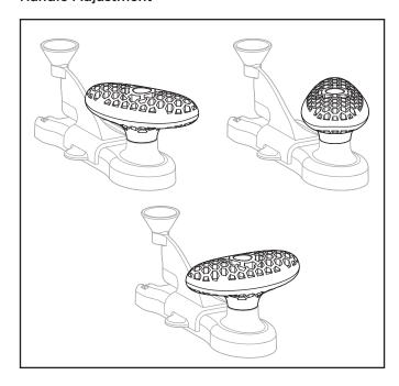
Handle is adjustable and can be loosened and rotated using a 3/16" hex tool to a comfortable position for the user.
