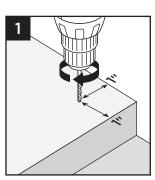
For best results using an 18V or higher cordless drill and the included HEXSTIX® depth setter, install fasteners at a 90° angle (perpendicular to the board). Drive the screws into the decking until the bit releases from the screw.
