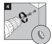
NOTE: Drive the screw in all at once, do not stop. You will hear the sound change when the screw is fully driven. Do not overdrive screw.
