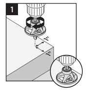
depth setter in a 18v or greater drill or impact driver, install fasteners at a 90° angle (perpendicular to the board). Drive the screws into the decking until the bit releases from the screw.
