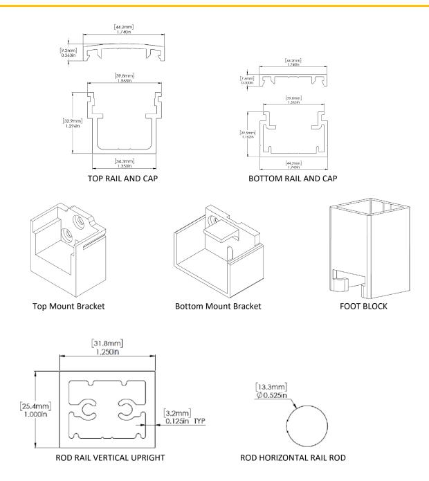
FIGURE 6 – SIGNATURE ROD RAILING SYSTEM COMPONENTS
