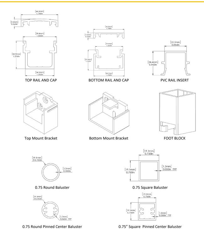
FIGURE 5 – SIGNATURE RAILING SYSTEM COMPONENTS
