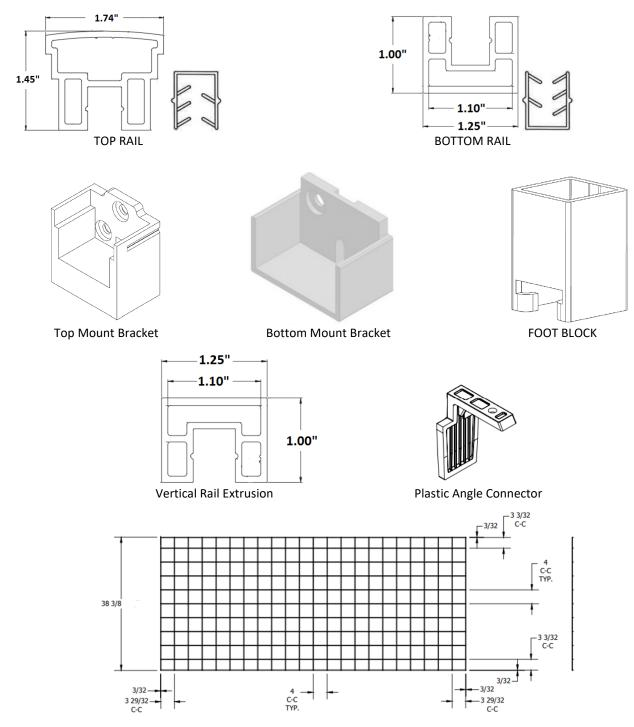
FIGURE 8 – SIGNATURE MESH RAILING SYSTEM COMPONENTS
