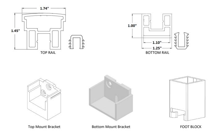
FIGURE 7 – SIGNATURE GLASS RAILING SYSTEM COMPONENTS
